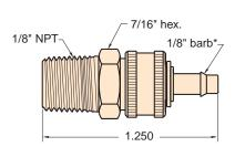
Minimatic® J-Series quick connect fittings are very compact yet provide a high flow of 14 scfm @ 100 psig. The electroless nickel plated brass body is available with #10-32 threads (M or F), 1/8" NPT threads (M or F), 1/4" NPT threads (M) or a 1/8" hose single barb configuration that is ideal for use with Clippard 3814-6 polyurethane hose.
